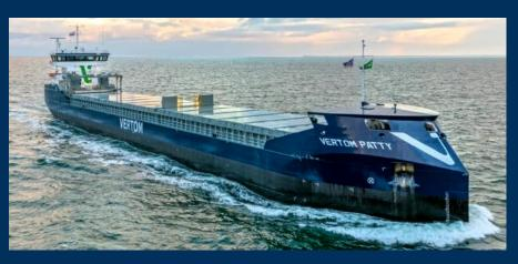
The LABRAX design was developed to Vertom's requirements and to provide both a highly efficient ship as well as one with versatility in its cargo operations. The completely box-shaped cargo holds ensure optimal loading flexibility and maximum cargo intake. The vessel is capable of grain or bale loading and
