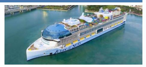
above the bridge. This glass and steel structure was hoisted intact onto the ship at the Meyer Turku yard in Finland, and it was the largest ever single lift of its kind.
